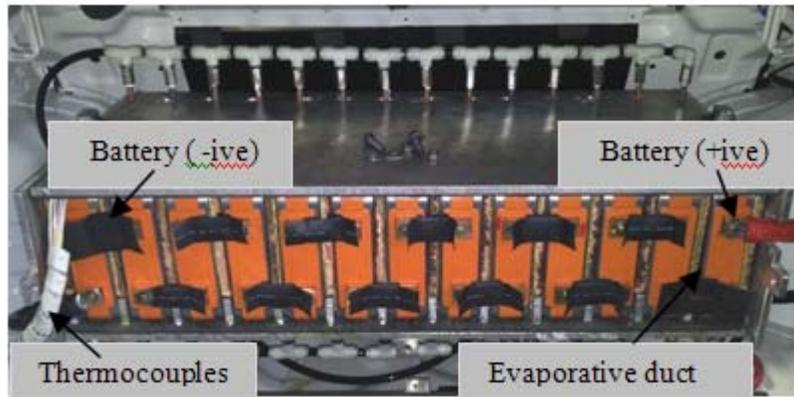
Figure 4: Evaporative Cooling System
