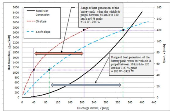
Figure 2: Battery cells heat generated without cooling
