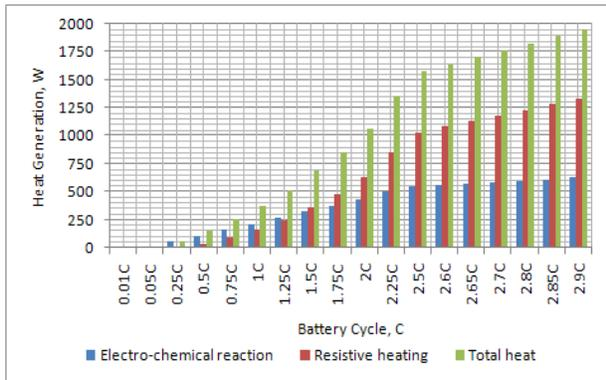
Figure 1 : Heat generation for the electrochemical reaction and resistive heating
