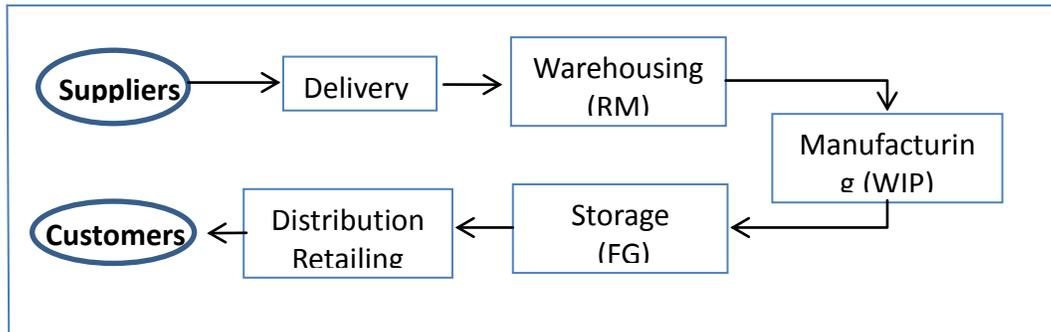
Figure 1: The main components in a supply chain
